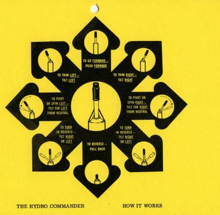
To go forward, move the Commander forward. The further you move it, the faster you go. To make a right or left hand turn, simply tilt the Commander to the right or left. Pull the Commander back to neutral and you brake to a stop. Whether you are moving straight ahead at the time of braking or in a turn, you brake both
